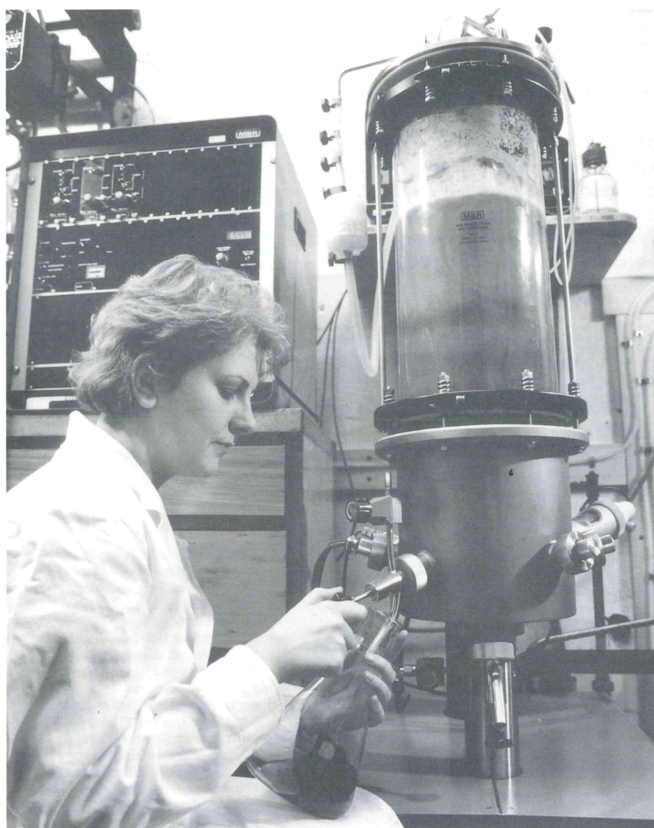
Pilot scale bioreactor used for growing micro-organisms. BTTG .
