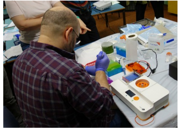
Brian Douglas demonstrates the loading of an agarose gel prior to electrophoresis
