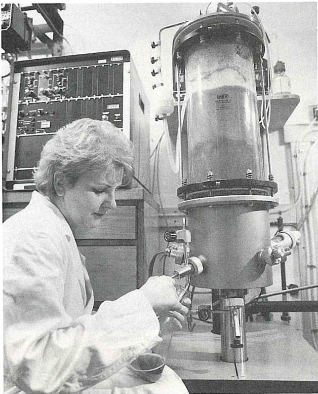
Figure 2. Pilot-scale 20 litre bioreactor.
