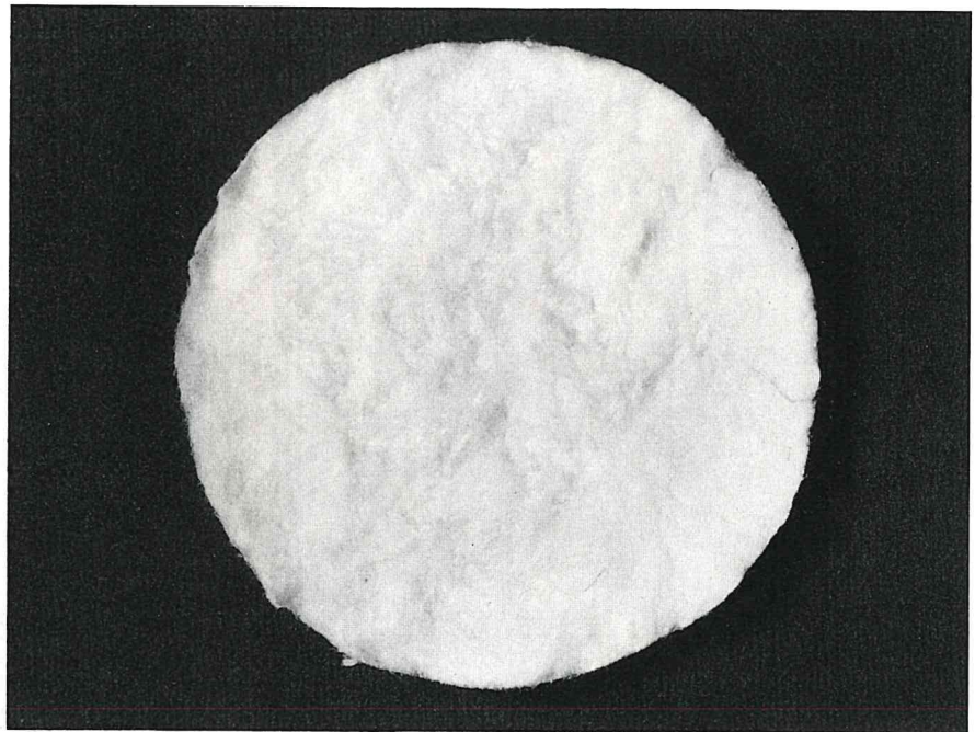
Figure 5. Absorbent pad composed of freeze-dried microfungal filaments.
