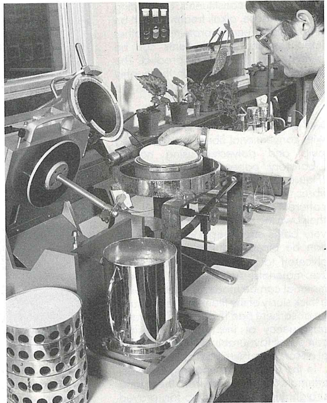
Figure 3. Preparation of wet-laid mats from microfungal filaments using a British Standard Sheet Paper-making Machine.
